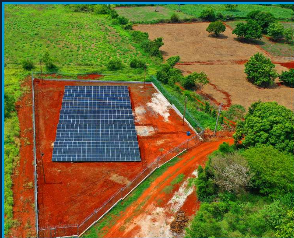
Beacon Little Park F3 pump station with 200 kW Solar PV system
